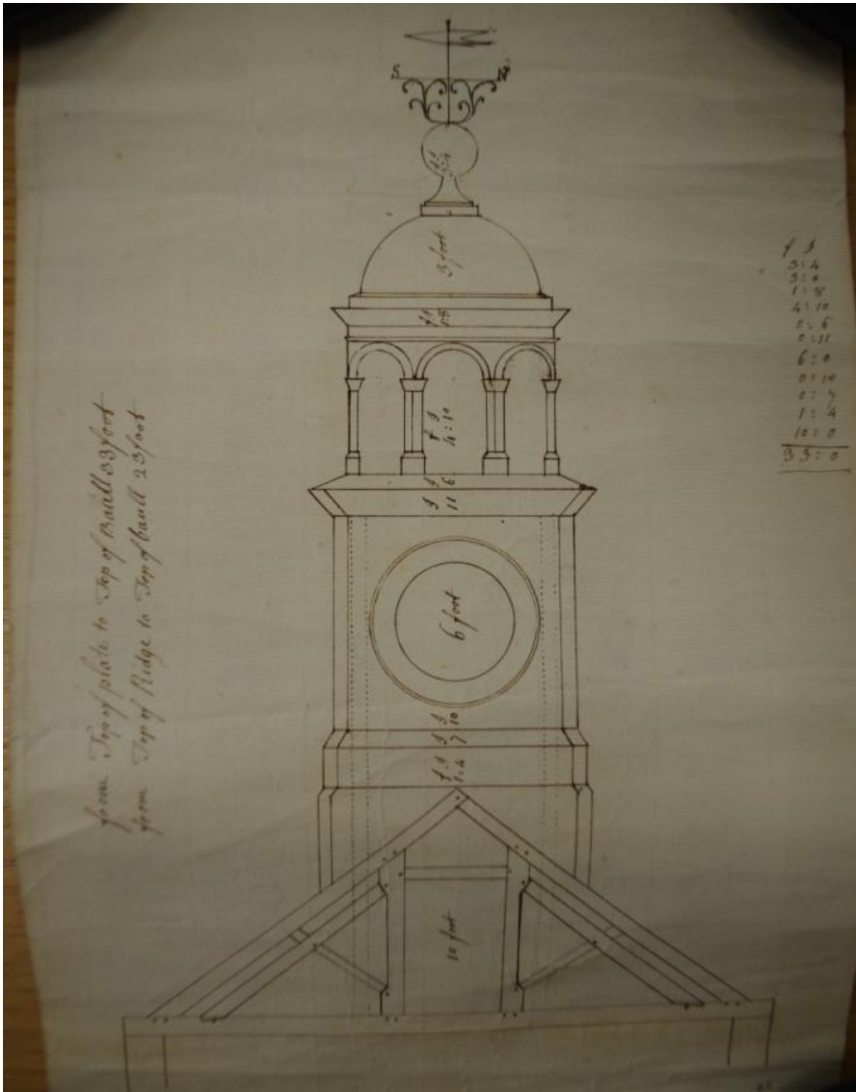
Figure 4 Architectural drawings and measurements for Amersham market hall and clock tower (c. 1682 - 1714).
